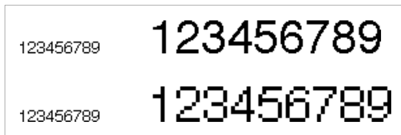
Figure 5-27 Scaled text and a scaled bitmap
